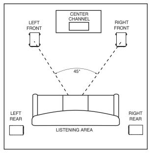
FIGURE 1 Typical Loudspeaker Placement
